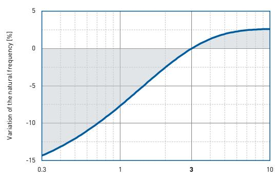
Correction values varying form factors specific load 0.15 N/mm<sup>2</sup>.
